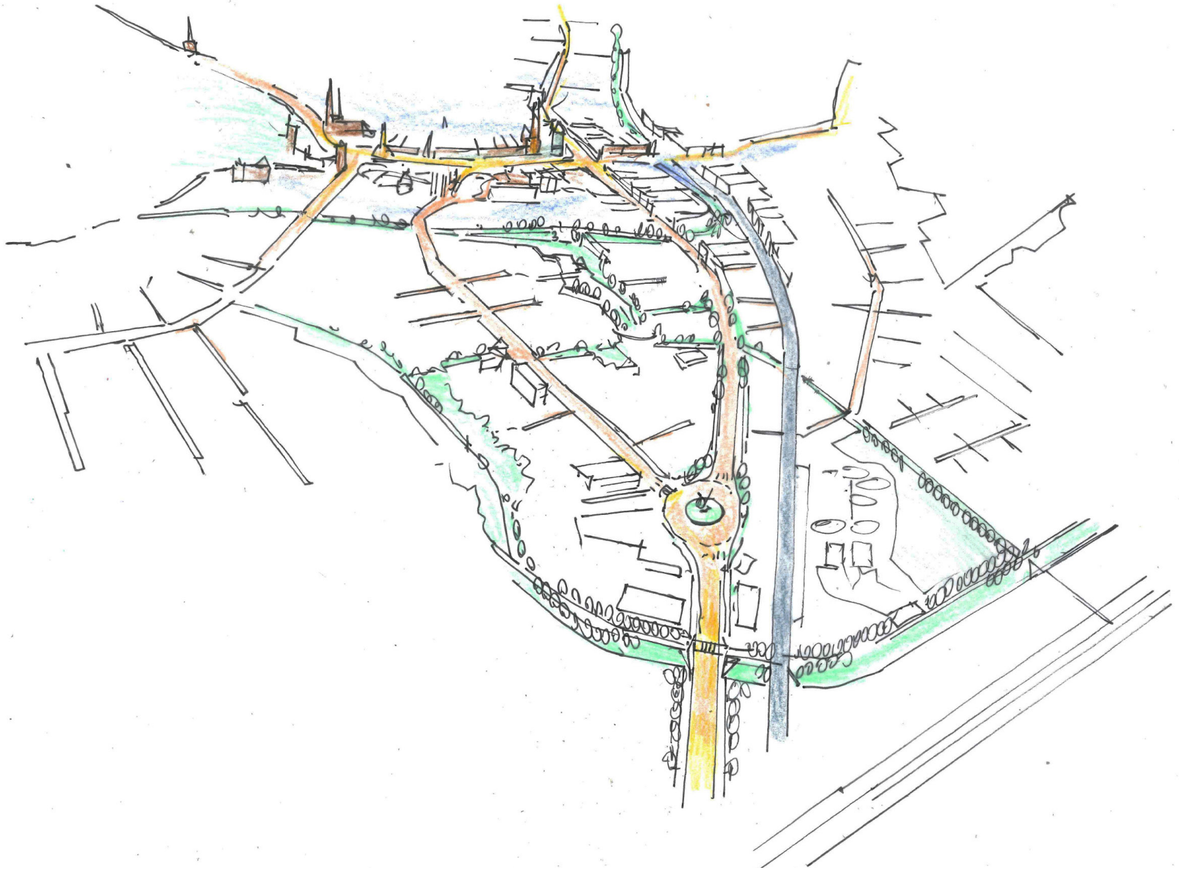
South Gateway: This aerial sketch of Northampton from the south illustrates how infrastructure improvements to the drainage structure and bike network might be strategically organized from the town-center, through a new open space and then to the city edge at the dike.
