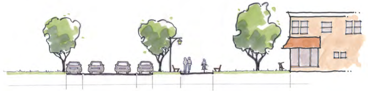
Proposed multiuse sidewalk section.
